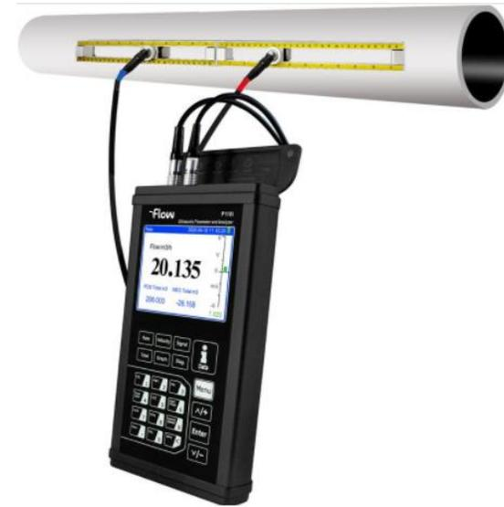
The portable hand-held flowmeter uses a universal transit-time technique, which can measure the time it takes for the ultrasonic signal to travel a known distance along the flow and the time it takes for another signal to propagate in the opposite direction to the flow to determine the velocity of the fluid being measured . The measurement is not restricted by the conductivity of the fluid, and has wider applicability compared with electromagnetic flowmeters.
